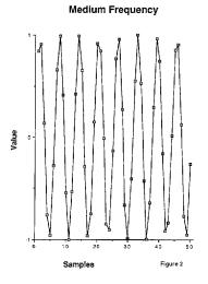
As the spatial frequency increases, the calculation of the MTF becomes nearly impossible as a shown on Figure 3. The problem is that the modulation has become a strong function of the phase of the cosine target relative to the sampling array.
